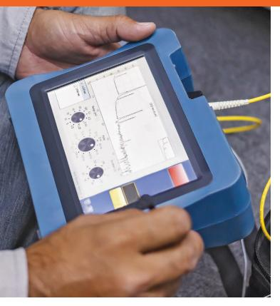
This two-day instructor-led course focuses on field testing and troubleshooting fiber optic spans/links and explains the various types of equipment and tools needed for acceptance testing, documenting performance, and finding problems in a fiber physical plant. The emphasis is on understanding proper OTDR settings, overall testing, and evaluating results.
